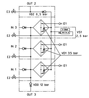
opening presseure of pressure difference valve: VD1 ∆pö 3,5 bar VD2 ∆pö 0.5 bar VD0 ∆pö 12,0 bar
